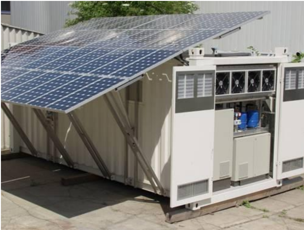
System for cooling and cold storing of milk
